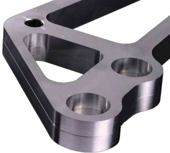
Clearly visible after the second machining: The deviation of 70 µm due to the thermal expansion of the ball screw drive
