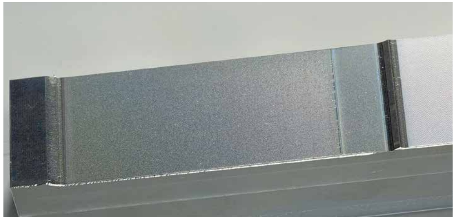
Figure 9: Milled surfaces: Rotary encoder 1 (above) with 3-fold greater interpolation error than rotary encoder 2 (below)
